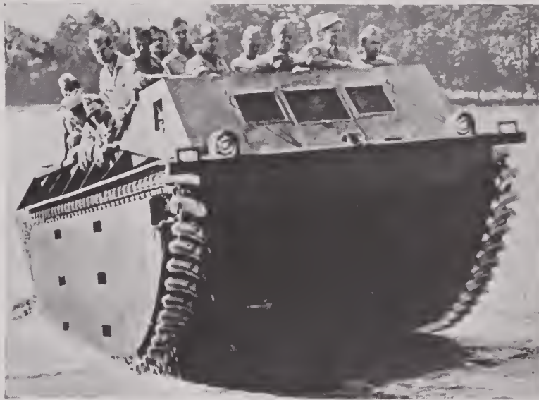
FIGURE 19. Early model of "Alligator" track-propelled amphibian representing "ground-up" design by John A. Roebling.
